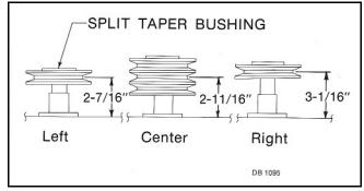
Figure 14. Belt Pulley Height Adjustments
